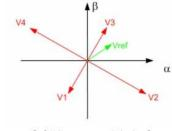
fig. 5 Voltage space vectors in the plan  $\alpha\beta$
