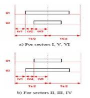
Fig.9 Pulse patterns for switching in the proposed method.
