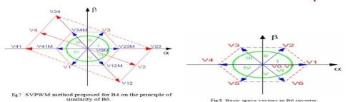
To simulate zero vectors of B6, we use the effective V0M
